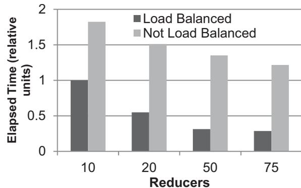
**Figure 4: Building an inverted index on skewed data ran 2x-4x faster with load balancing. Speedups increased as we increased the number of reducers (Experiment: 24 GB data; cluster #3; 1000 distinct words with a Zipf(1) word frequency distribution)**
