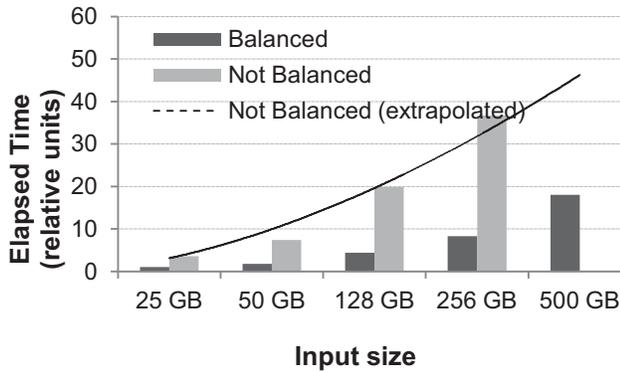
**Figure 3: Oracle Loader for Hadoop on skewed data ran 3x-4x faster with load balancing. Speedups increased with increasing input size. Without load balancing, the largest experiment of 500GB had not completed even after running for 3X longer than its balanced counterpart (outside the plotted region) and was killed (Experiment: OLH writing Datapump-format files to HDFS on cluster #3; 128 reducers; 128 reduce-keys (i.e. database partitions) with Zipf(1) skew)**
