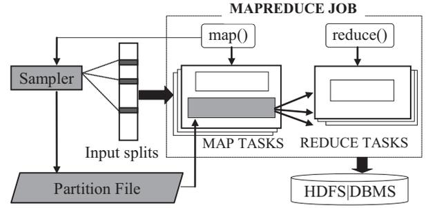
**Figure 1: Workflow of Hadoop jobs with load balancing.** The shaded boxes are new components added by our system. Our Partitioner replaces the job’s original Partitioner which is not shown in this figure.
